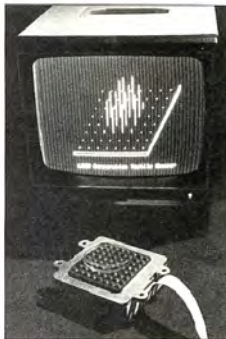
Robot touch sensor from 1985
